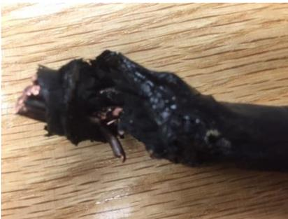
The Facilities and Services Electric Shop responded to a call at Myrna's Children's Village that electric service was lost at building. Upon investigation, the electricians discovered a damaged feeder cable. The crew removed the damaged section of cable and restored power to the building in less than 30 minutes.
